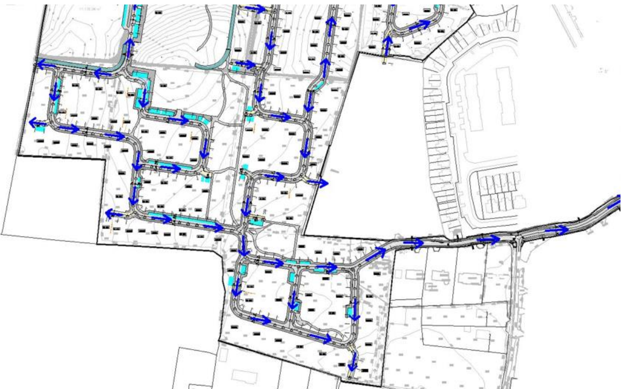
Figure 6.8. Proposed Overland Flow Route (Southern section).
