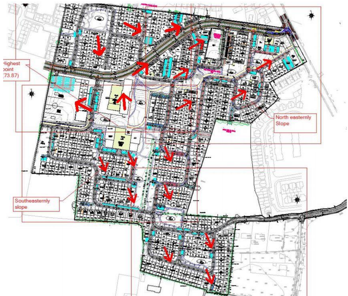
Figure 6.2. Existing Overland Flow Routes.
