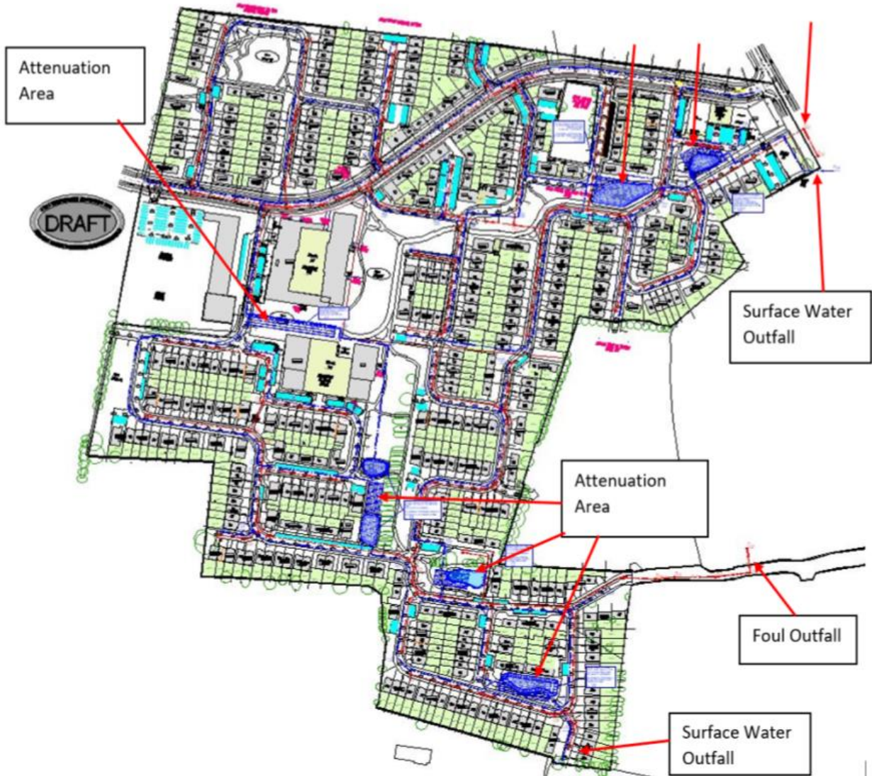
Figure 6.1. Proposed Foul and Surface Water Drainage Networks.
